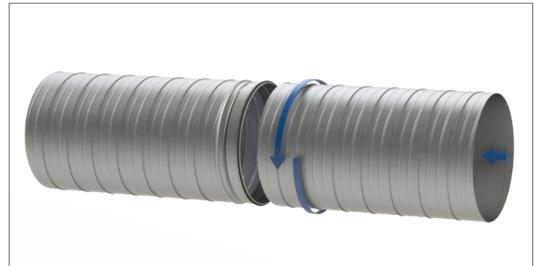
2.2. Preliminarily attach fittings to ducts on the floor. Turn and push components simultaneously to facilitate attaching.
