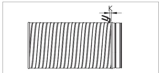
2.5. For saddling a saddle (NPSK-T or NPSV-T) is recommended, as this will enable connection without cutting apart a duct. Place the saddle on the duct and draw the saddle contour on the duct surface. Cut a hole into the duct about 10 mm smaller than the contour. Start cutting from the centre hole of the area to be cut. Apply a sealing compound on hole edges before attaching the Saddle. Place the saddle in the correct position and attach.
